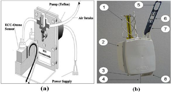
(Source: Thompson *et al.*, 2011) Figure 1: Ozonesonde and radiosonde RS292 used over Nairobi
