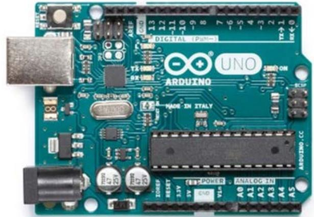
Fig. 6. Arduino Uno microcontroller [16]
