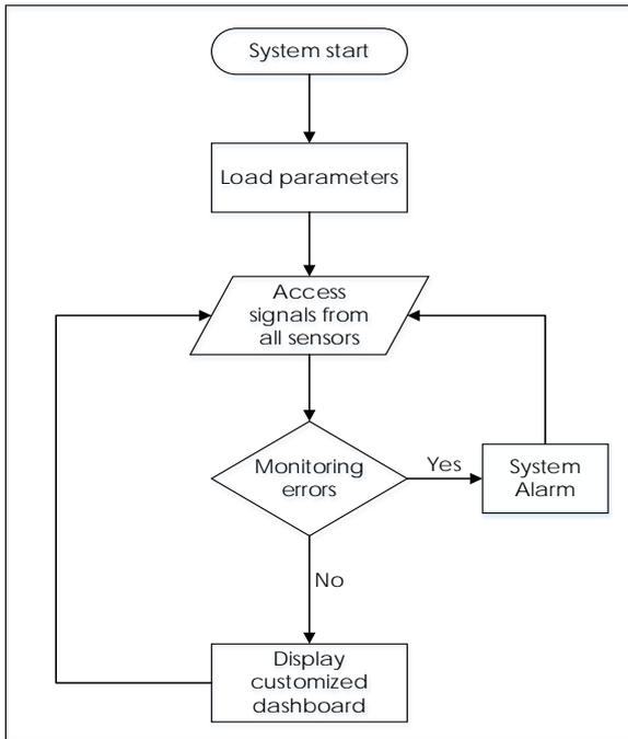
Fig. 8. Operation flow diagram
