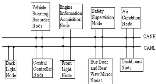
Fig. 3. The Controller Area Network [7]
