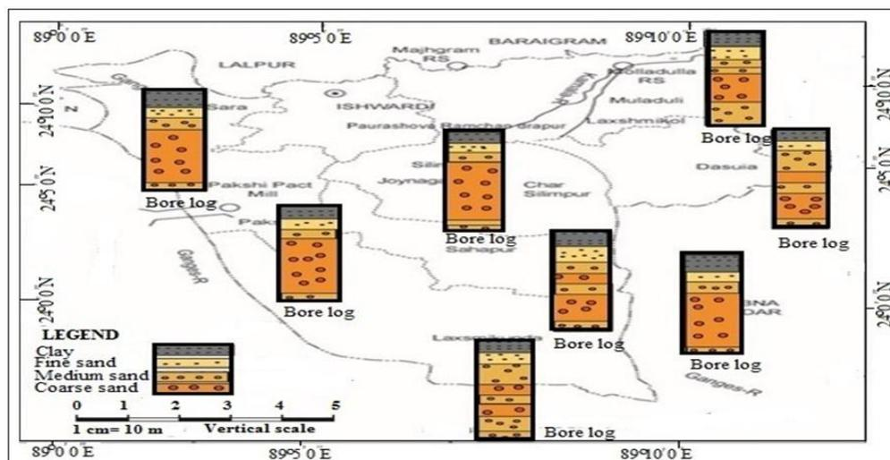
Fig. 2. Vertical cross-section of sub-surface lithology of the study area
