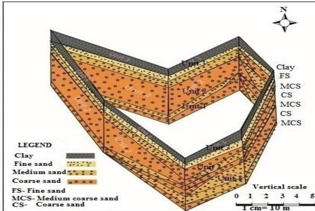
Fig. 3. Panel diagram shows the geological profile of the study area
