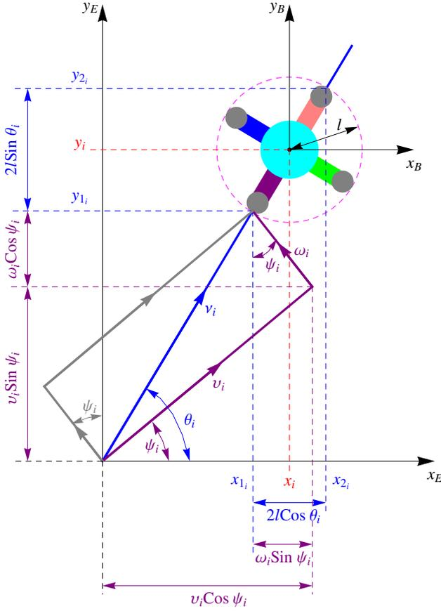
Fig. 1. Kinematic model of a Quadrotor UAV.
