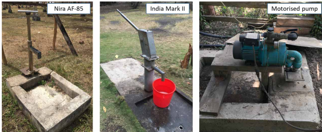
Figure 2 | Pump types included in the assessment.
