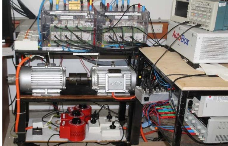
Figure 3: Experimental rig of the IM electrical drive
