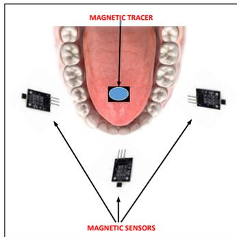
Fig. 6. Sensor placement for TDS
