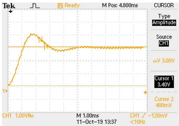
Fig. 10. The controlled output from the DC-DC buck converter using FOPI
