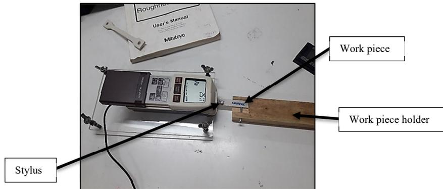
Fig. 3. Surface roughness measurement set-up.
