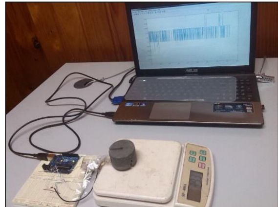
Figure-8. Calibration of force sensor in real time.
