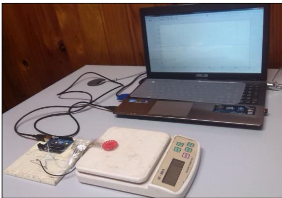
Figure-6. FSR interfaced using Arduino Uno and MATLAB (with puck for calibration).
