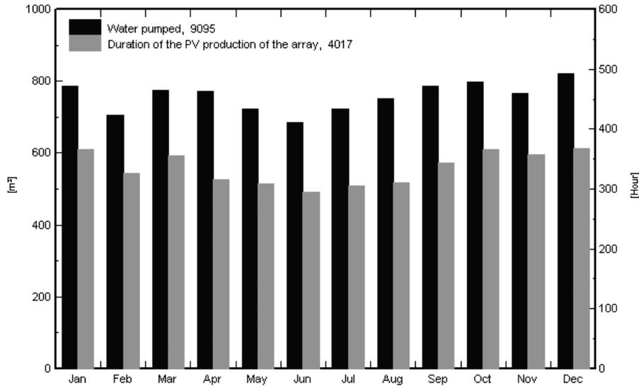
**Fig. 3.** System performance: Water pumped and PV production
