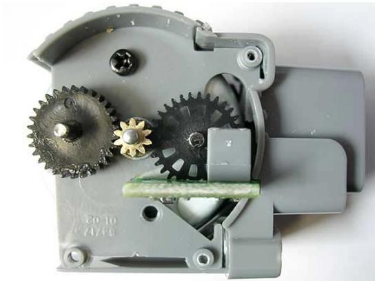
Figure 13-NXT Motor Exploded View Showing Encoder and optical fork
