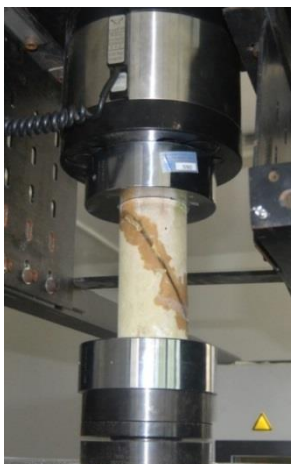
Figure 7. Adhesive joints composed of cylindrical masonry blocks bonded by an epoxy-hybrid adhesive.
