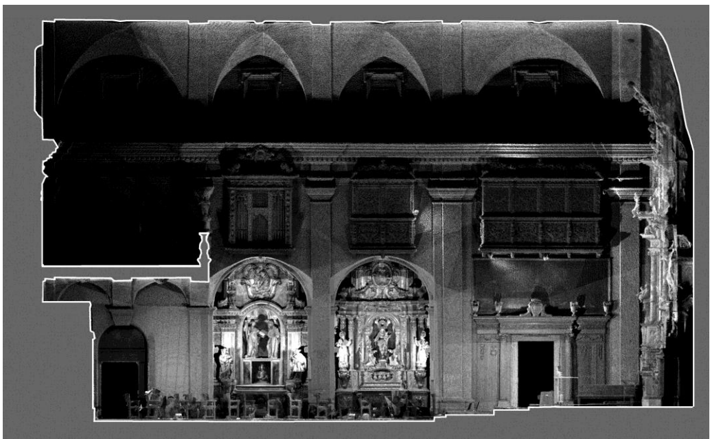
Figure 3. Architectural section obtained by laser scanning.
