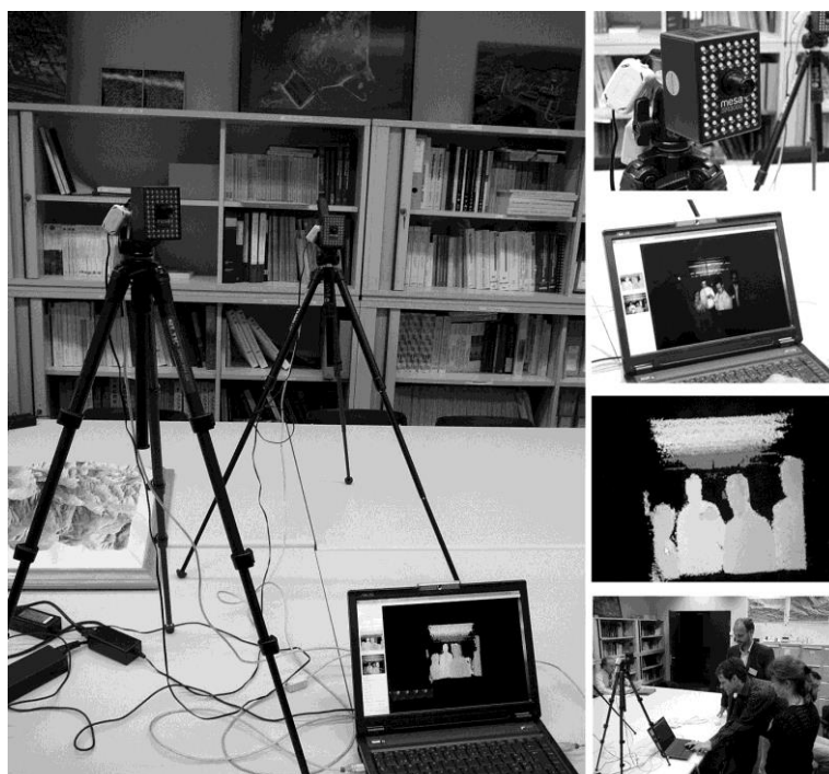
Figure 10. A 3D camera and the result of the grey-image capture and representation of distance.
