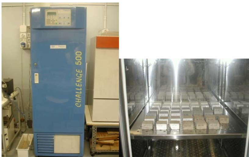
Figure 12. A climatic chamber and some samples inside.
