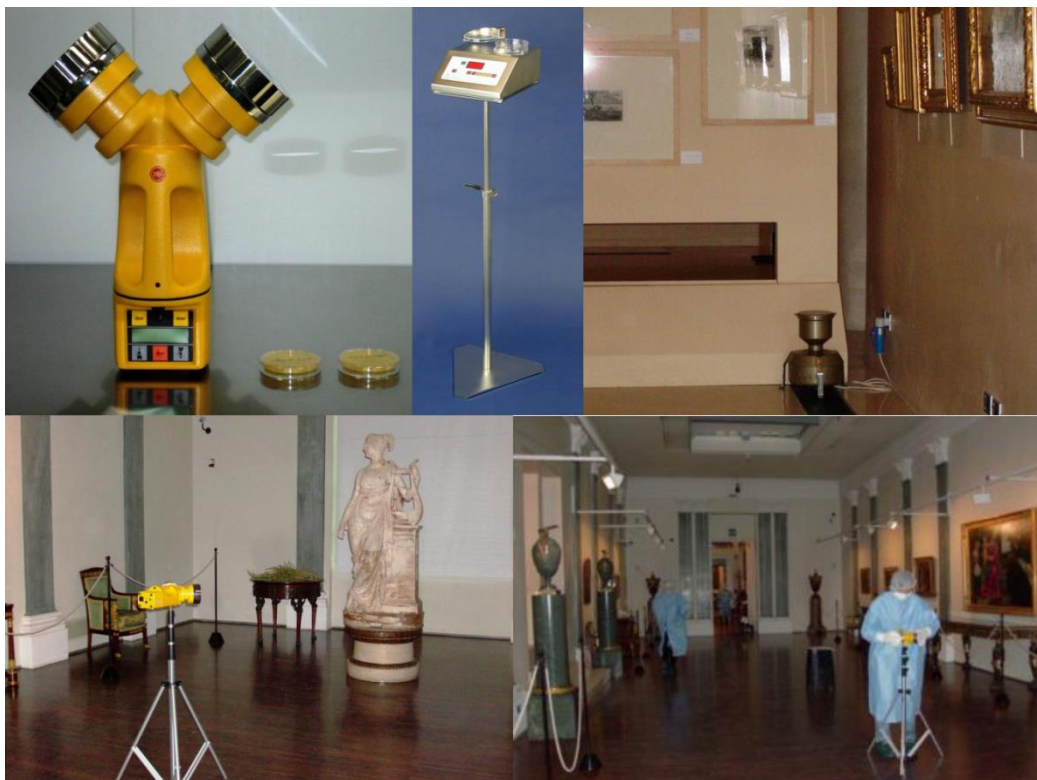
Figure 2. Equipment for air sampling. a) Active sampler; b) Passive sampler; c) Hirst spore trap; d) and e) Two rooms of the Magnani Rocca Foundation during air monitoring.
