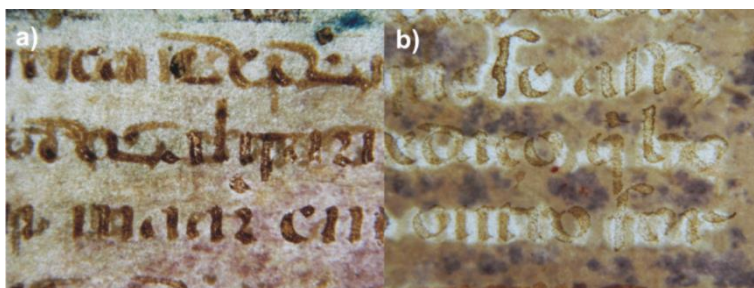
Figure 4. Picture under transmitted light taken from the foral charter of Sintra showing Fe based ink a) Fe and Zn based ink b).
