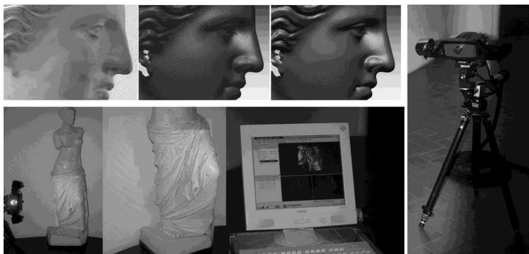
Figure 4. Top: original model, TIN and virtual model. Bottom: data capture, targets and light pattern.
