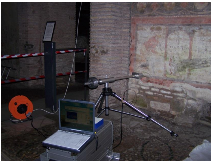
Figure 2. Portable unilateral NMR instrument measuring the moisture content in the wall painting Saint Clement at mass and the legend of Sisinnius in St. Clement's Basilica, Rome.
