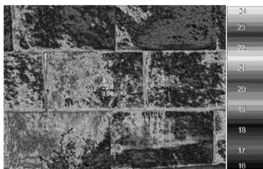
Figure 13. Part of the Roman wall in Barcelona, captured by a thermal camera.
