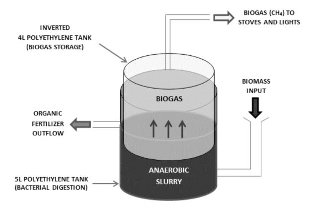
Figure 2: Schematic of a typical domestic anaerobic digester for biomass designed in the context of renewable energy projects in Pacific Islands such as Tuvalu and Fiji.
