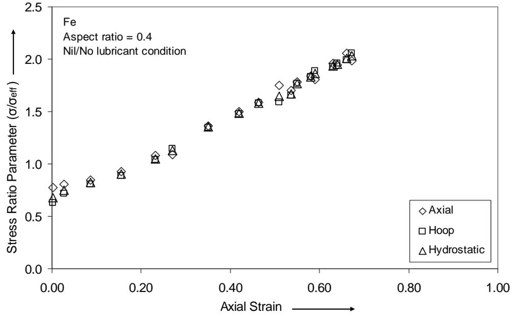
Fig. 10: Variation of stress ratio parameter ( $\sigma_{\theta} / \sigma_{eff}$ ), ( $\sigma_m / \sigma_{eff}$ ) and ( $\sigma_z / \sigma_{eff}$ ) against axial strain.
