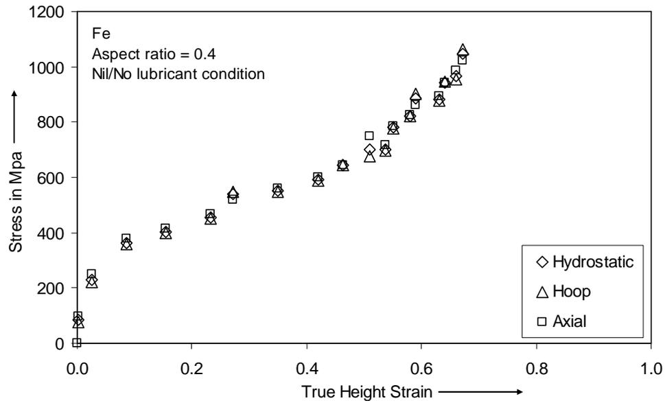
Fig. 5: Variation of hydrostatic, hoop and axial stresses against true height strain.
