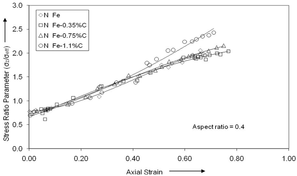
Fig. 9: Variation of stress ratio parameter,  $\sigma_z / \sigma_{eff}$  against axial strain.
