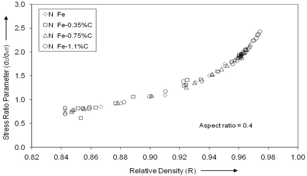
Fig. 7: Variation of stress ratio parameter,  $\sigma_z / \sigma_{eff}$  against relative density.
