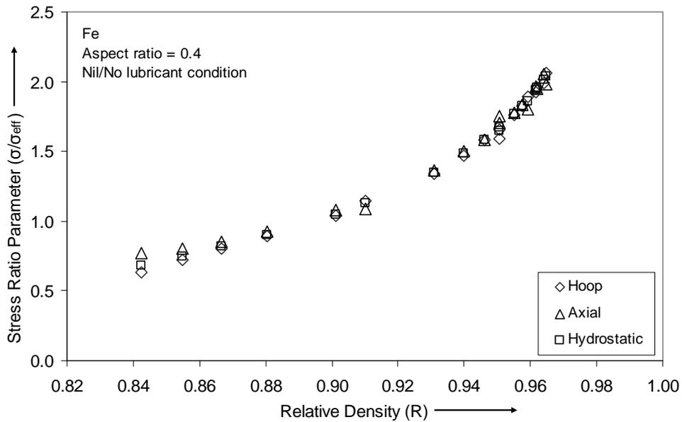
Fig. 8: Variation of stress ratio parameter ( $\sigma_\theta / \sigma_{eff}$ ), ( $\sigma_m / \sigma_{eff}$ ) and ( $\sigma_z / \sigma_{eff}$ ) against relative density.
