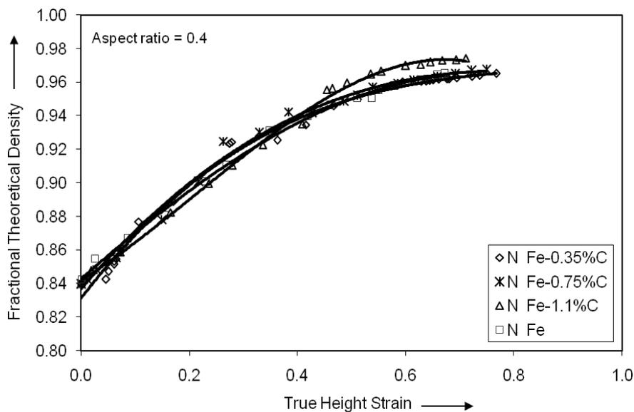
Fig. 3: Relationship between fractional theoretical density and true height strain.
