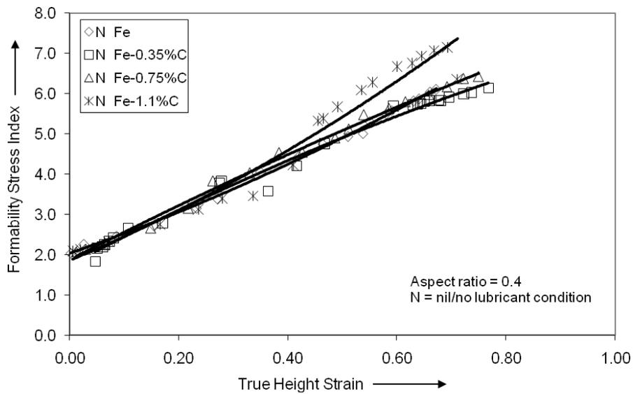
Fig. 1: Relationship between formability stress index and true height strain.
