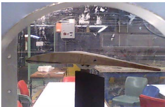
Fig. 5. A model of USPB_01 airfoil mounted on the wind tunnel
