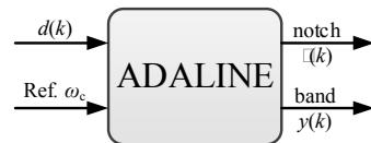
Fig. 2. Schematic representation of the neural adaptive filter.
