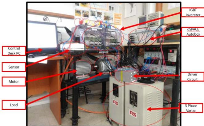
Figure 7: Experimental rig
