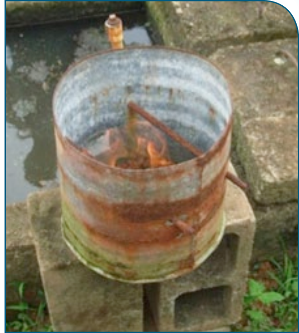
Figure 11: Biogas energy from pigs' waste - targeting zero emission from integrated farming at Monfort Boys Town, Veisari : Photo by Joeli Veitayaki
