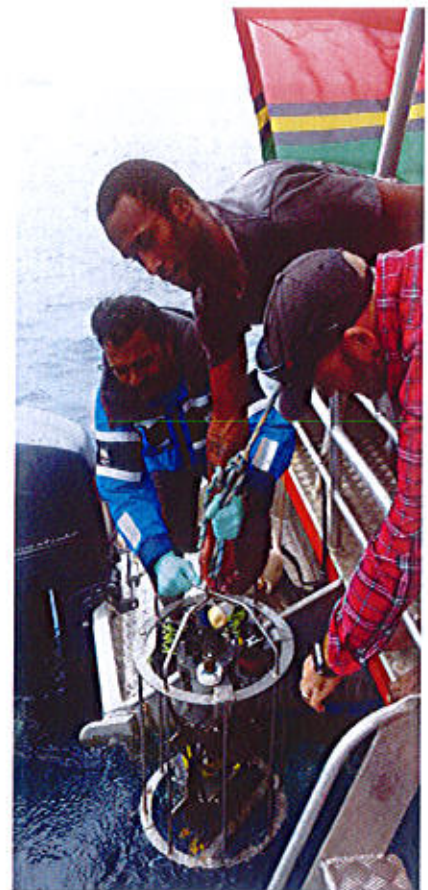
Sampling with the profiler measuring salinity, temperature, light and chlorophyll at depth.
