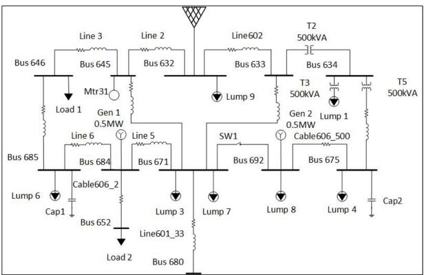
Fig. 2 Mesh Network Modeled in ETAP
