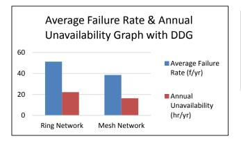
Fig. 3 Average Failure Rate & Annual Unavailability Graph with DDG
