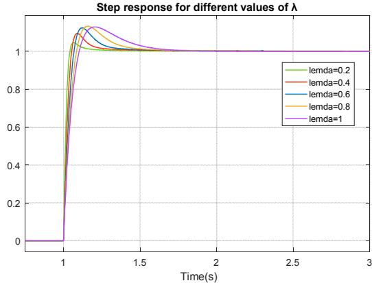
Figure 5: Step response of a FOPI controlled 1<sup>st</sup> order system
