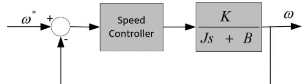
Figure 1: Simplified speed loop
