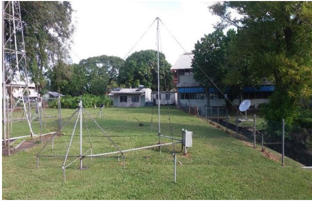
A snapshot of local field trip: showing VLF magnetic loop and GNSS antennas used to record the data: Pictures taken from a section of field trip report of a PH302 student. April 2018.
