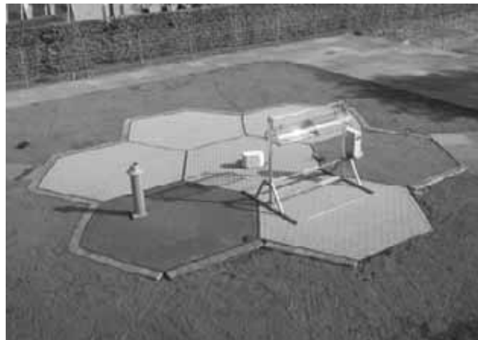
Test field near Muenster for evaporation measurements on different (waterpermeable) pavement systems.
