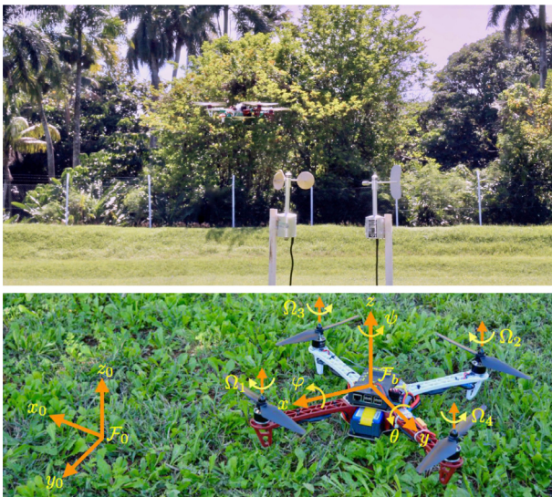
Fig. 1. An Erlecopter aircraft and the anemometer, used to collect ground truth information about the wind speed (then converted to wind force), during testing at the University of South Pacific (Fiji) campus (above). The aircraft with associated coordinate frame (below).
