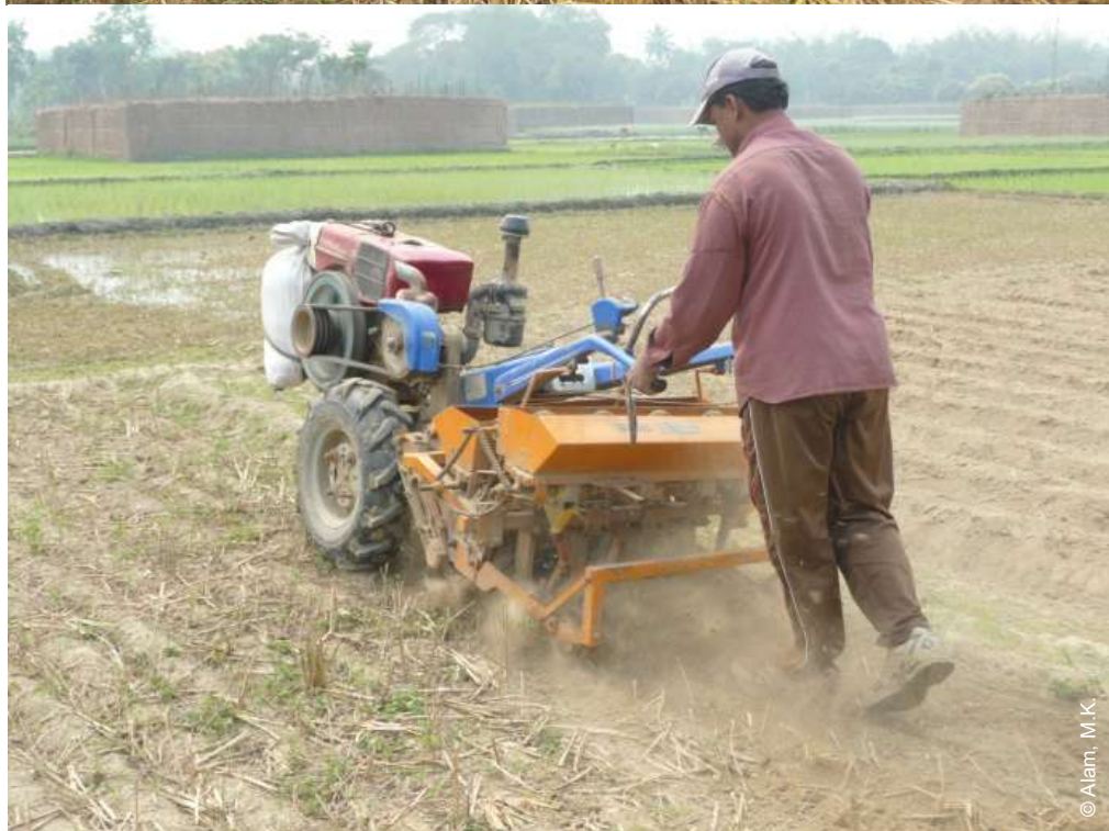
Photo 30. Two-wheel tractor with Versatile Multi-crop Planter (VMP), sowing through standing residue retained at higher rate at Digram, Rajshahi (top) and low rate (bottom) at Alipur, Durgapur, Rajshahi, Bangladesh
