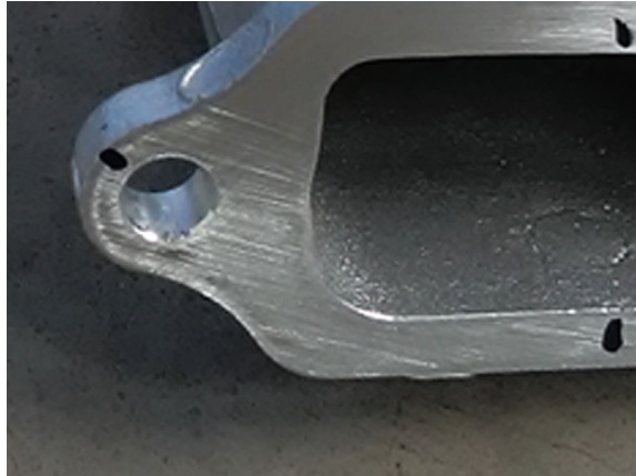
Fig. 5 Rubbing marking on the face of manifold
