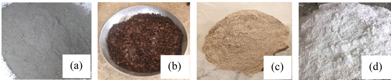
Fig. 1. Binding materials used (a) PLC, (b) Shea nutshells, (c) VPA, and (d) CP.
