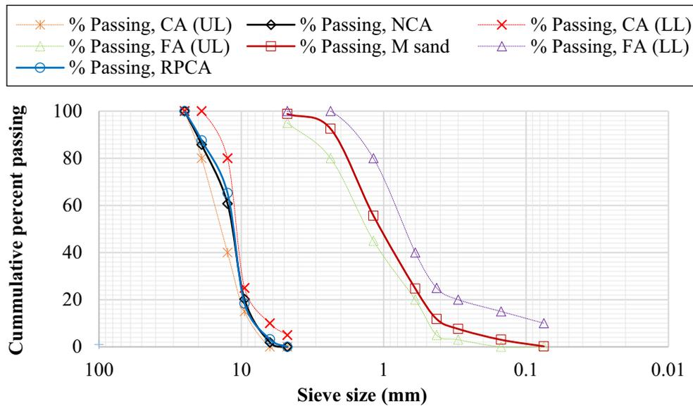
Notes: CA and FA connote coarse aggregate and fine aggregate; UL and LL represent the upper limit and lower limit
