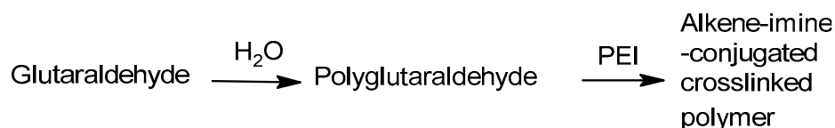
Scheme 2. Proposed crosslinking mechanism of polyethylene imine with glutaraldehyde [34].
