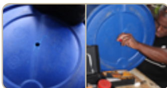
Figure 22: Left: Drain out (22 mm). Right: Inserting the \frac{3}{4} inch valve and sealed with silicon to prevent any leakages.
