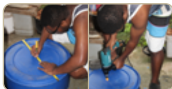
Figure 21: Left: Marking out the centre of the bin. Right: Drill a hole at the centre using 22 mm in diameter drill bit.
