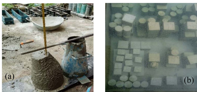
Fig 3. Experimental operations showing (a) the slump test and (b) the curing of concrete samples.
