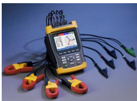
Figure 3: Fluke 434 3-phase power quality analyser.
