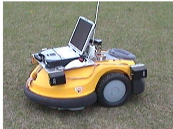
Figure 1: Mowing robot “Robomower”.
