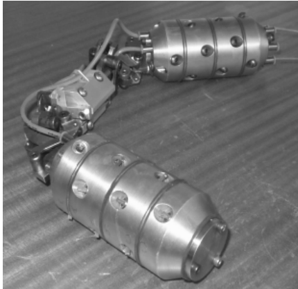
Figure 3: Pipeline robot using Hood-Kowski joint.
