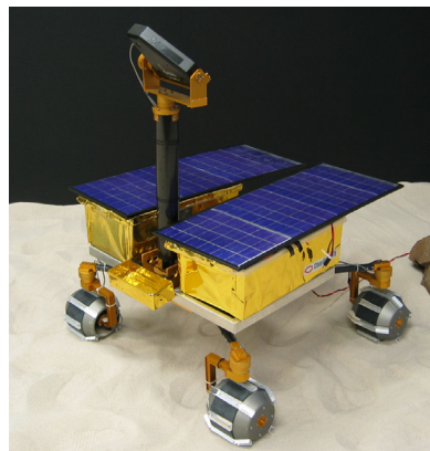
Figure 1: Micro5-05 rover test-bed system.
