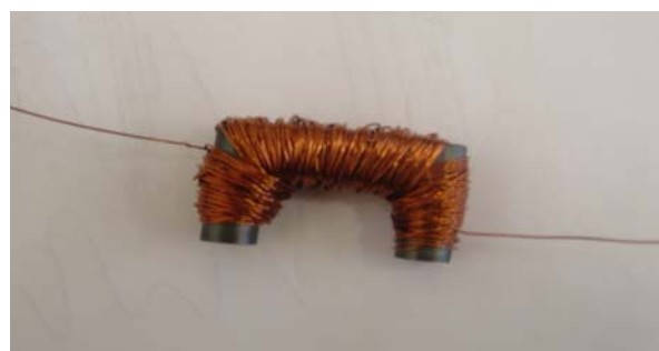
Figure 19: A typical pickup coil.
