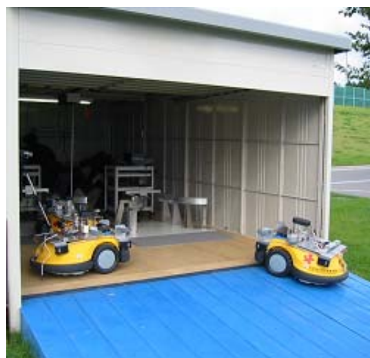
Figure 4: Mowing robots and charge station.
