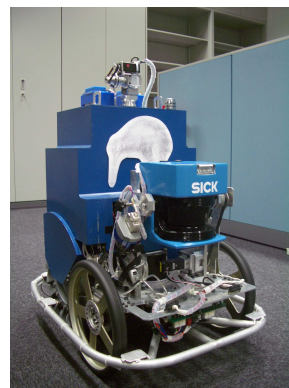
Figure 1: The mobile robot platform with a front mounted SICK laser range sensor which can be rotated about it's horizontal axis.
