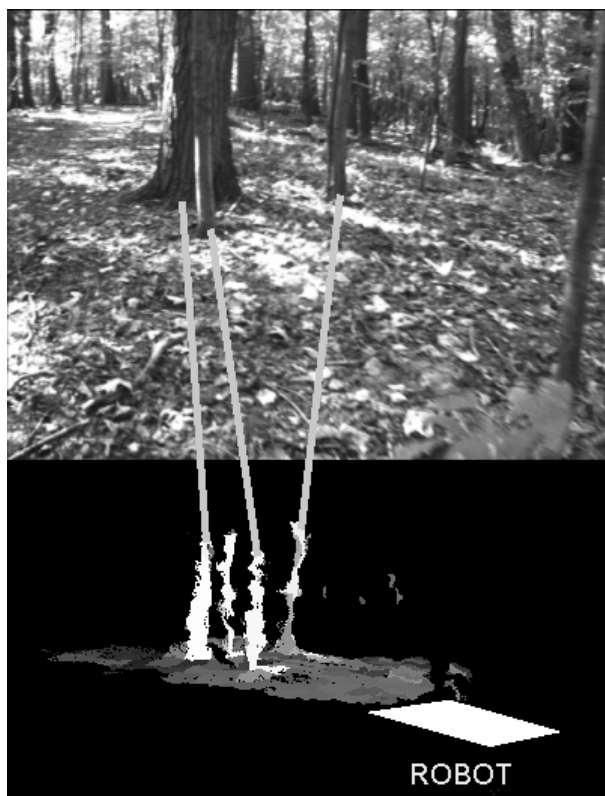
Figure 9: Correspondence between scene and greyscale encoding of cost for 3D data.
