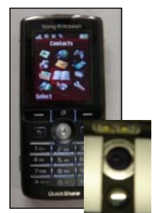
Figure 5: K750i and its (inset) 2.0 mega pixel camera located on the back plane.
