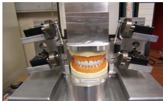
Figure 1: Prototype chewing robot at Massey University, New Zealand.
