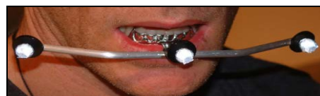
Figure 5: Custom made brace for jaw tracking with six degrees of freedom.
