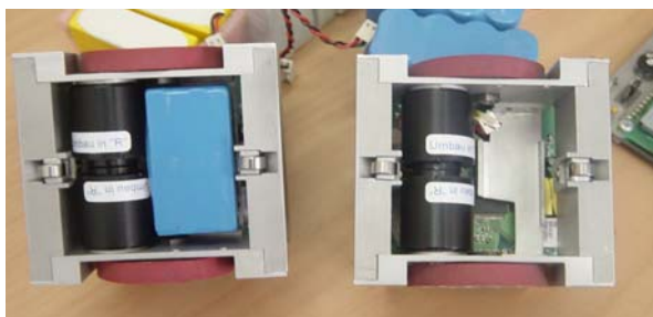
Figure 4: The battery inside a soccer robot.
