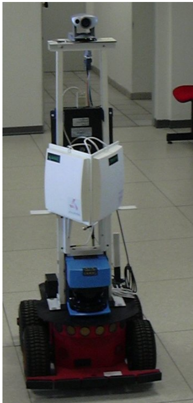
Figure 2: Pioneer 3AT platform equipped with Sick laser range finder, RFID reader and two antennas.
