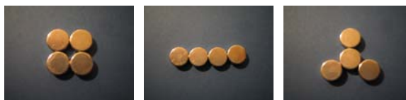
Figure 2: The three stable two-dimensional formations of magnetic discs: grid (left); chain (centre); and triangular (right).
