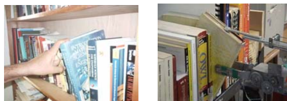
(c) Human finger and Probe pull back. Downward force and friction present have the effect of prying the book out of the shelf.
