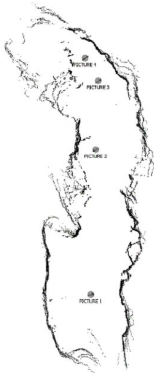
Figure 3: 2D map of the explored area of the cave obtained after the application of the scan-matching algorithm. The explored corridor is about 40x5m 2 .
