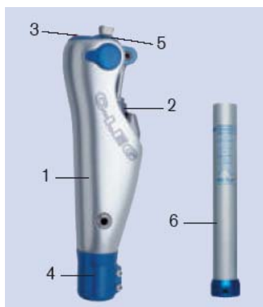
Figure 5: C-leg: knee-inspired structure design + mechanical components + electronics.
