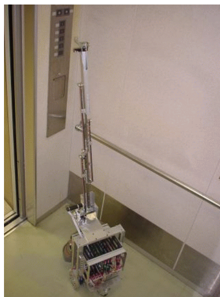
Figure 10: Pushing an elevator button.
