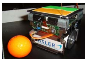
Figure 3: A MiroSot robot: prototype with a local camera.
