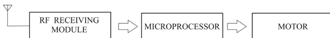
Figure 6: Diagram of the robot's onboard electronic system.
