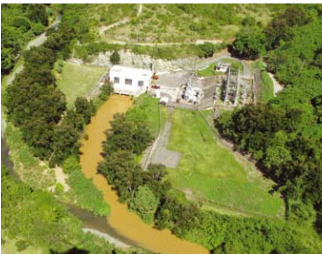
This shows unintended damage from large scale engineering modification of catchment areas in Puerto Rico. Drainage from a nearby catchment area was diverted into the Guanica Bay Rio Loco catchment to improve water flows and generate electricity; however, sediments from the modified catchment have damaged some of the best reefs in Puerto Rico. These sediments have washed off steep hillsides (right) cleared for sun grown coffee (Case Study 7).
