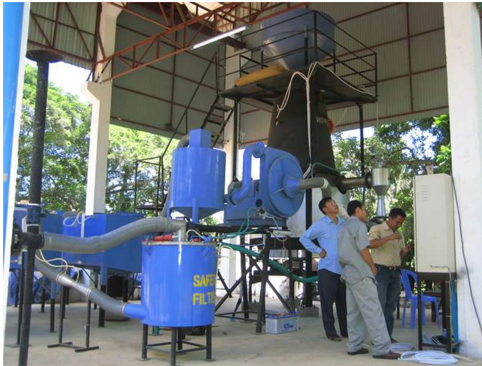
Biogasification system; Source: Energy Summit – Samoa presentation
