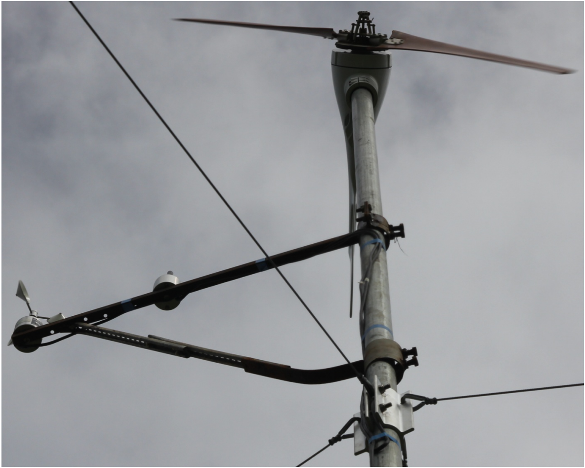
Fig. 7 Close-up view of the Air-X turbine with the 2-bladed rotor and anemometer setup
