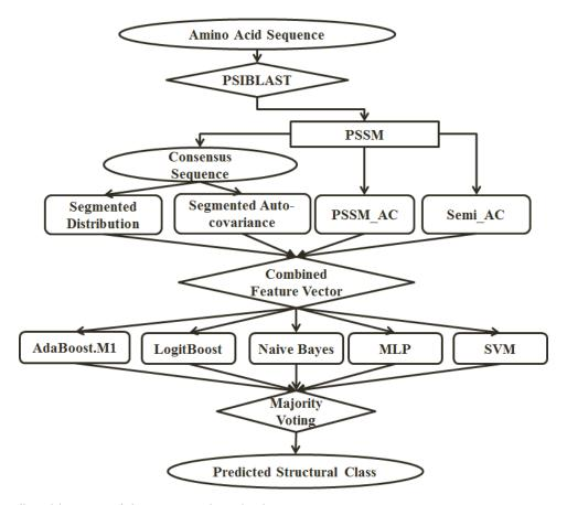
Fig. 2. The overall architecture of the proposed method.
