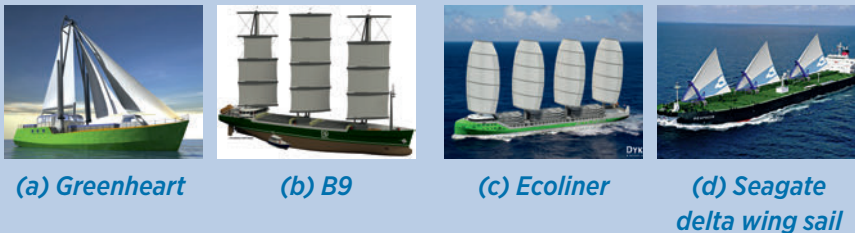
Figure 2: Examples of ship designs deploying soft-sail technology
