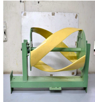
Fig. 5: Gorlov experiment model
